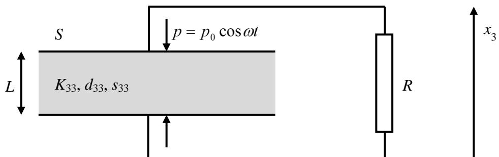
In the following, we first consider the equivalent electric scheme shown in the figure above and obtain relation between  $E_3$  and  $D_3$  in real variables; after that we will generalize the result to complex variables.
